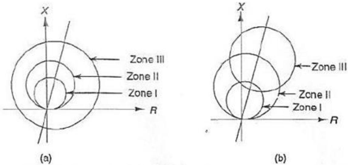
**FIGURE 8.15** (a) Mho and offset mho relays for transmission lines (b) Mho and offset Mho relays for long lines
