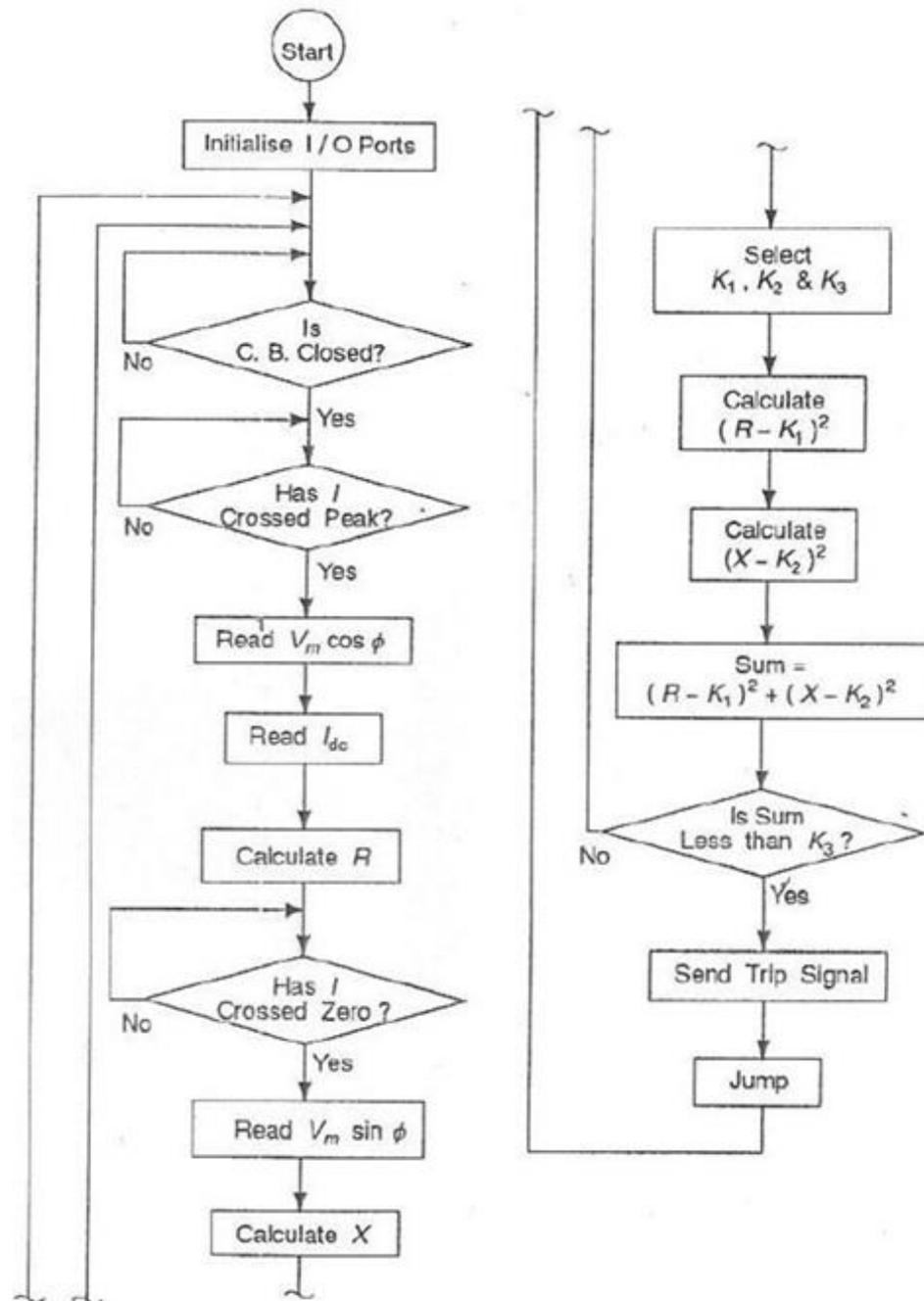
FIGURE 8.22 Program flowchart for offset mho relay
