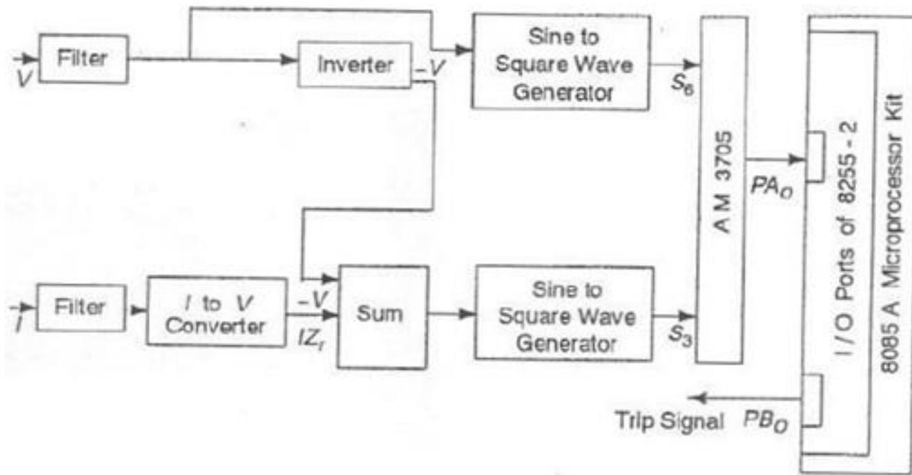
(c) Schematic diagram of interface
