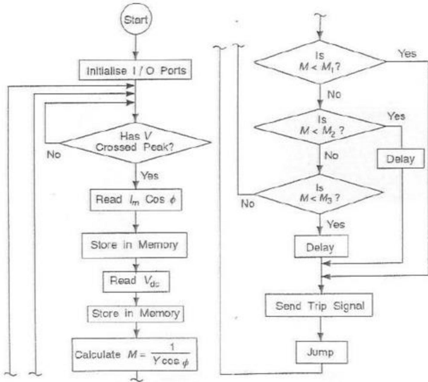
FIGURE 8.19 Program flowchart for mho relay
