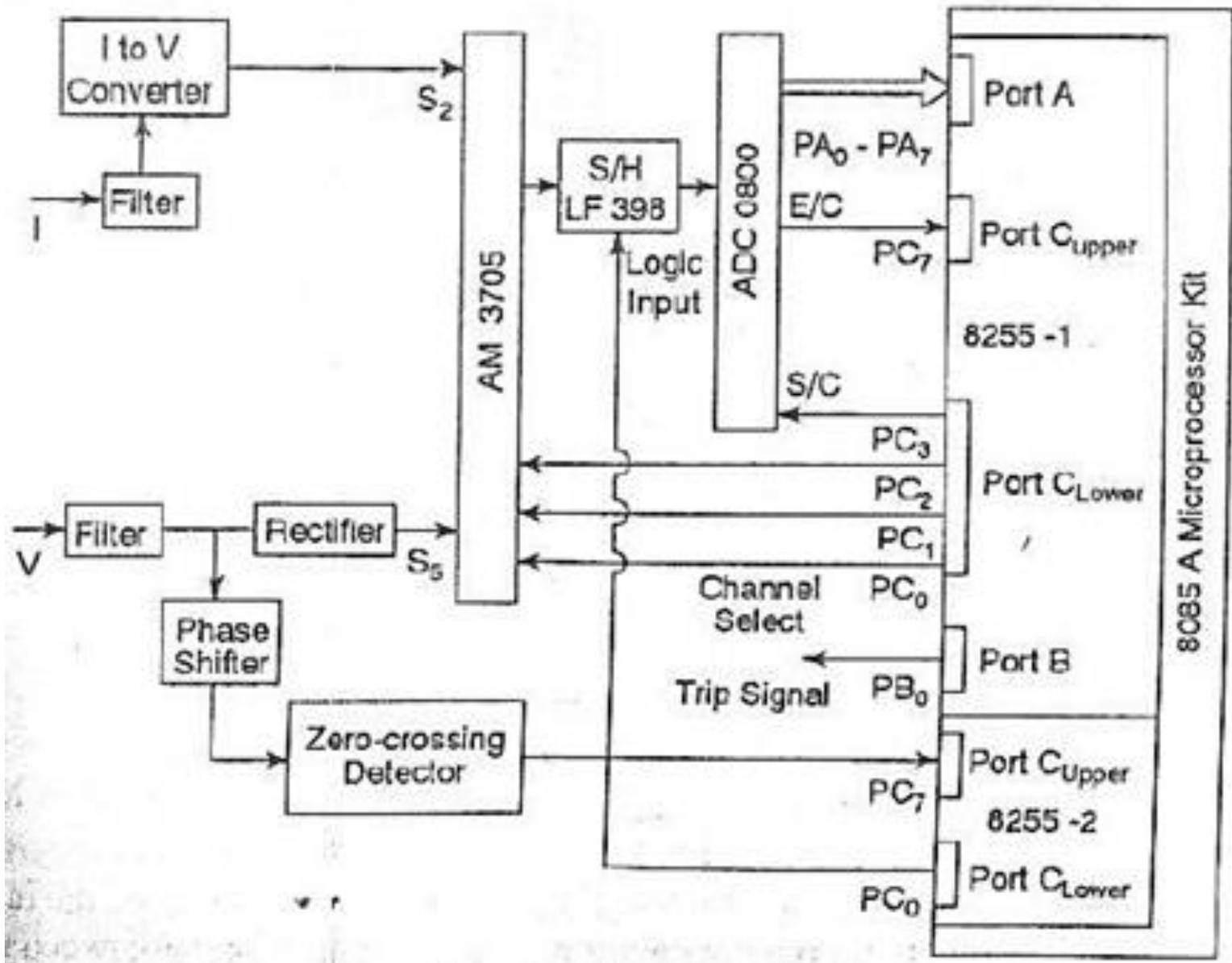
FIGURE 8.18 Block schematic diagram of interface for mho relay
