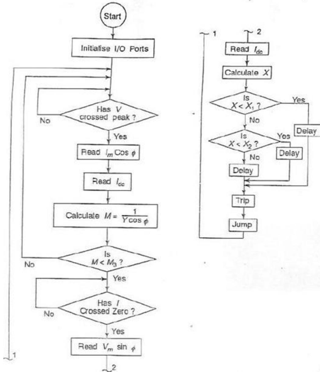
FIGURE 8.11 Program flowchart for reactance relay
