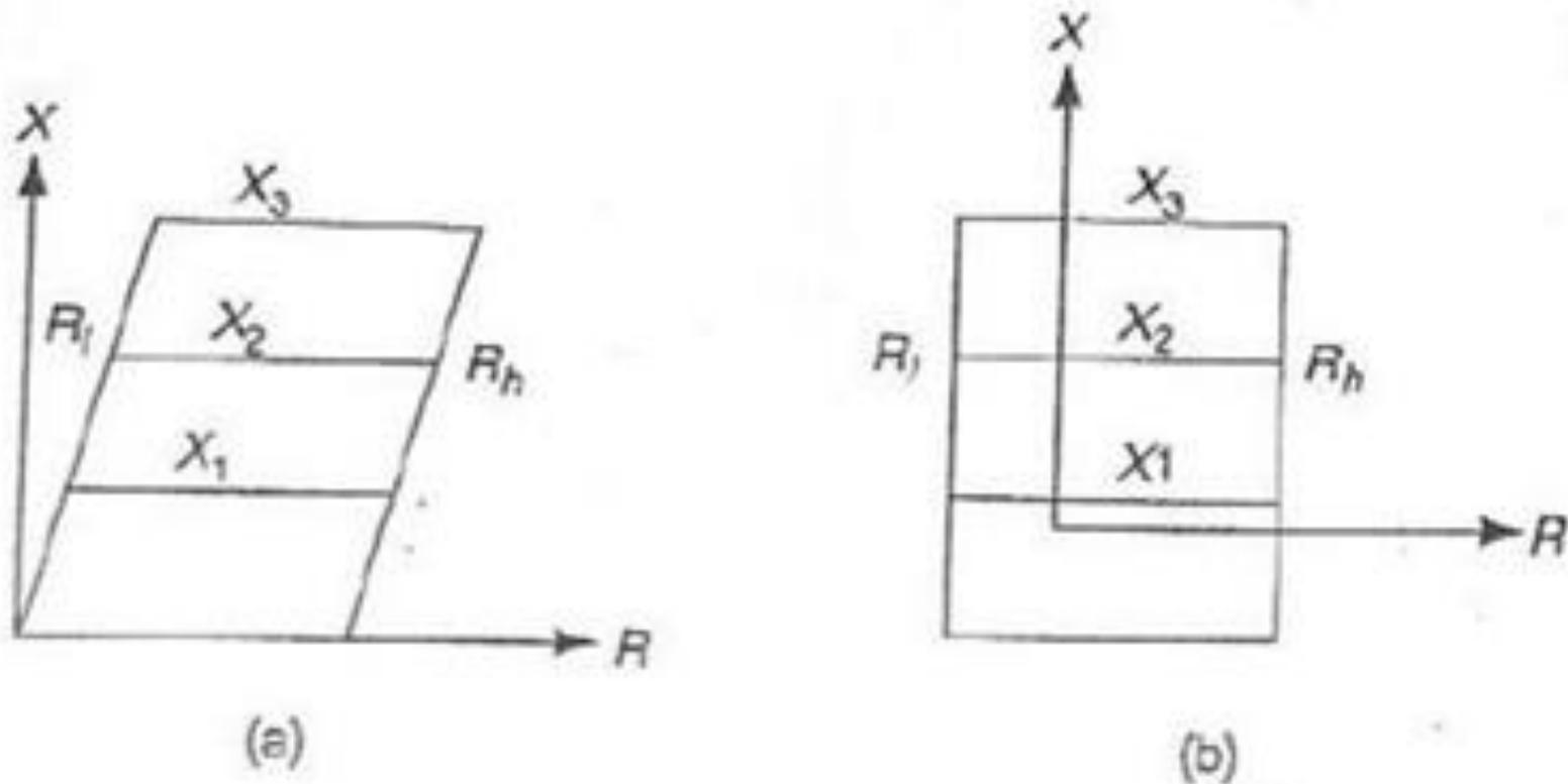
FIGURE 8.24 (a) Quadrilateral relay passing through origin
