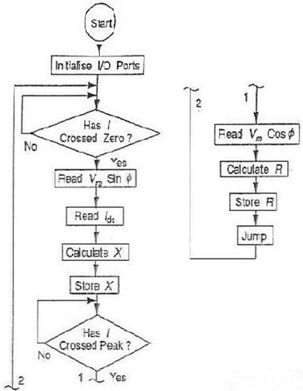
FIGURE 8.14 Program flowchart for measurement of  $R$  and  $X$
