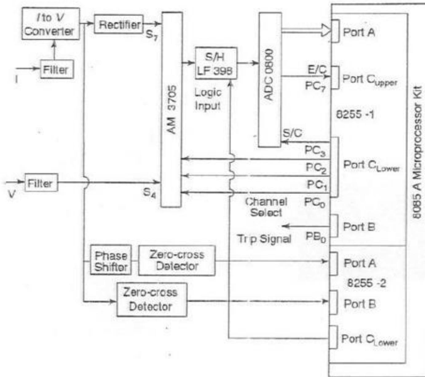
FIGURE 8.21 Block schematic diagram of interface for mho, offset mho, restricted mho and quadrilateral relays
