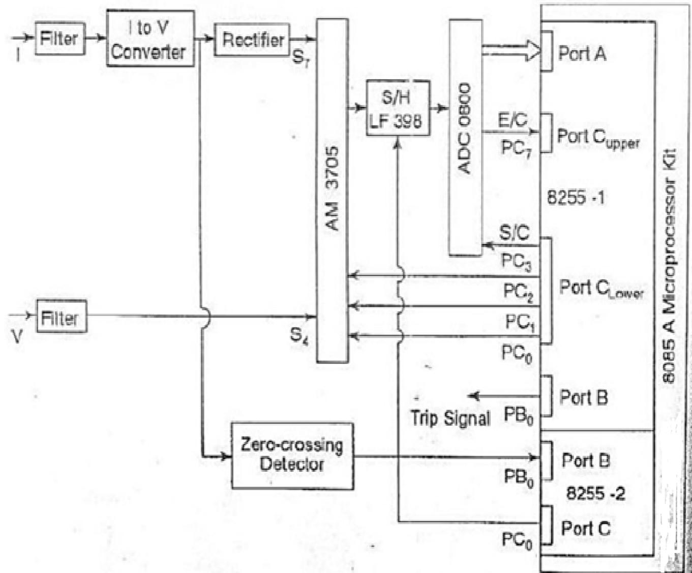
FIGURE 8.9 Block schematic diagram of interface for reactance relay
