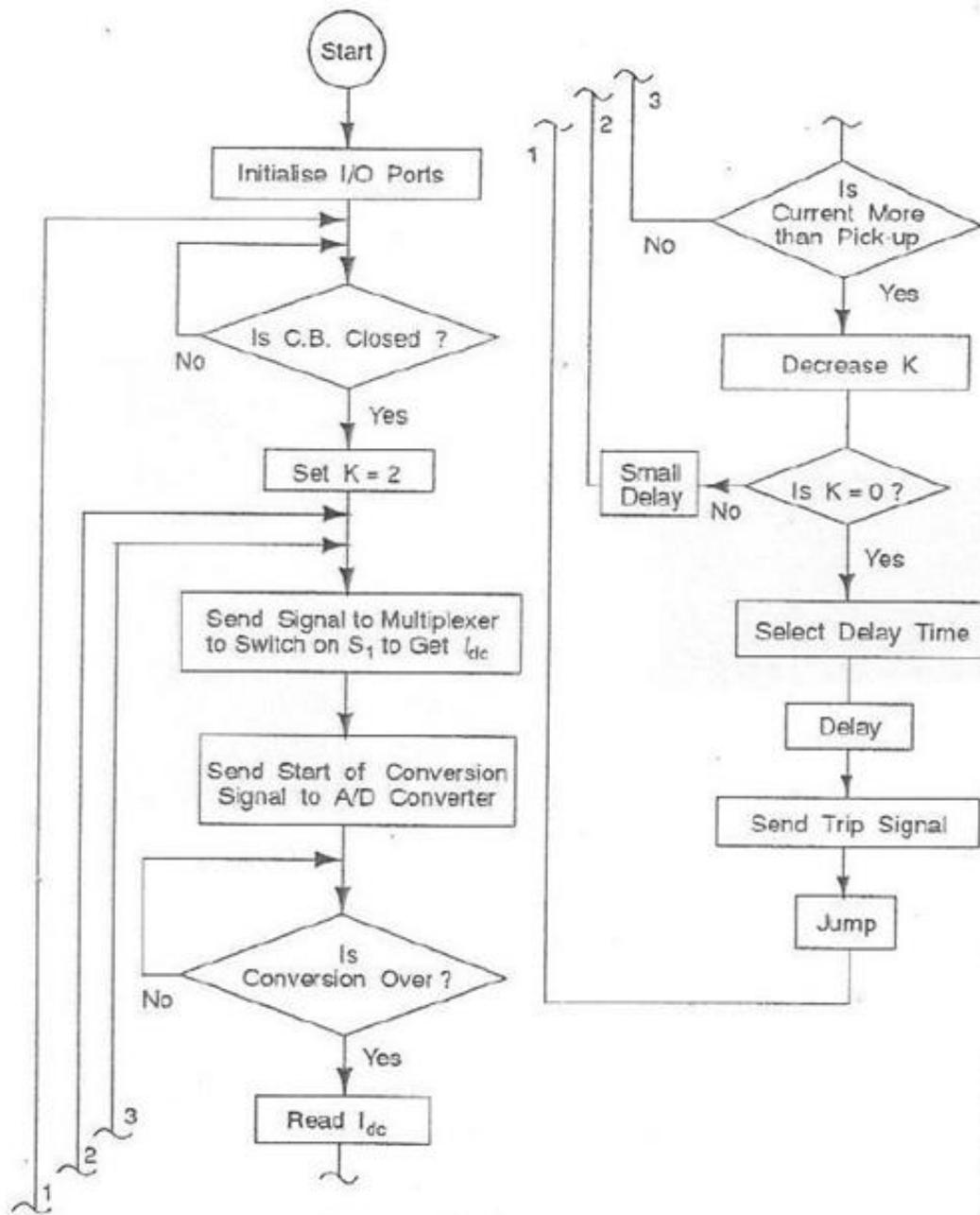
FIGURE 8.2 Program flowchart for overcurrent relay
