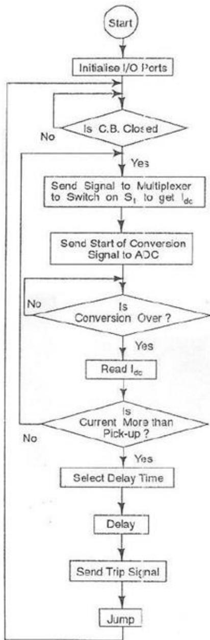
FIGURE 8.1(b) Program flowchart for overcurrent relay
