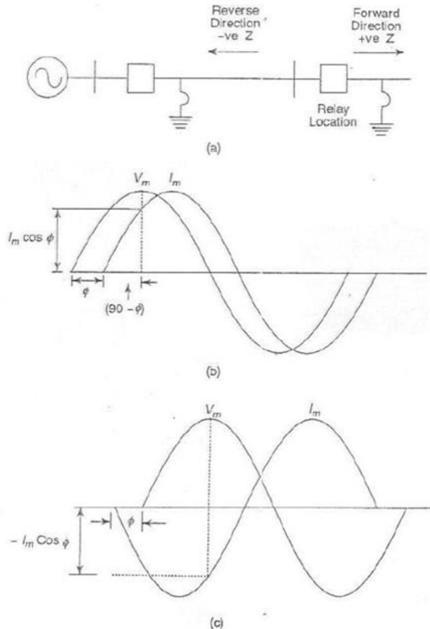
FIGURE 8.5 (a) Location of directional relay (b) Instantaneous value of current at peak voltage (c)  $I_m \cos \phi$  for fault in reverse direction
