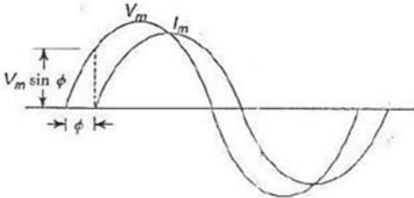
FIGURE 8.8 Instantaneous value of voltage at current zero
