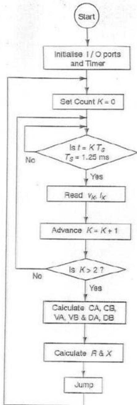
FIGURE 8.27 Program flowchart for computation of  $R$  and  $X$
