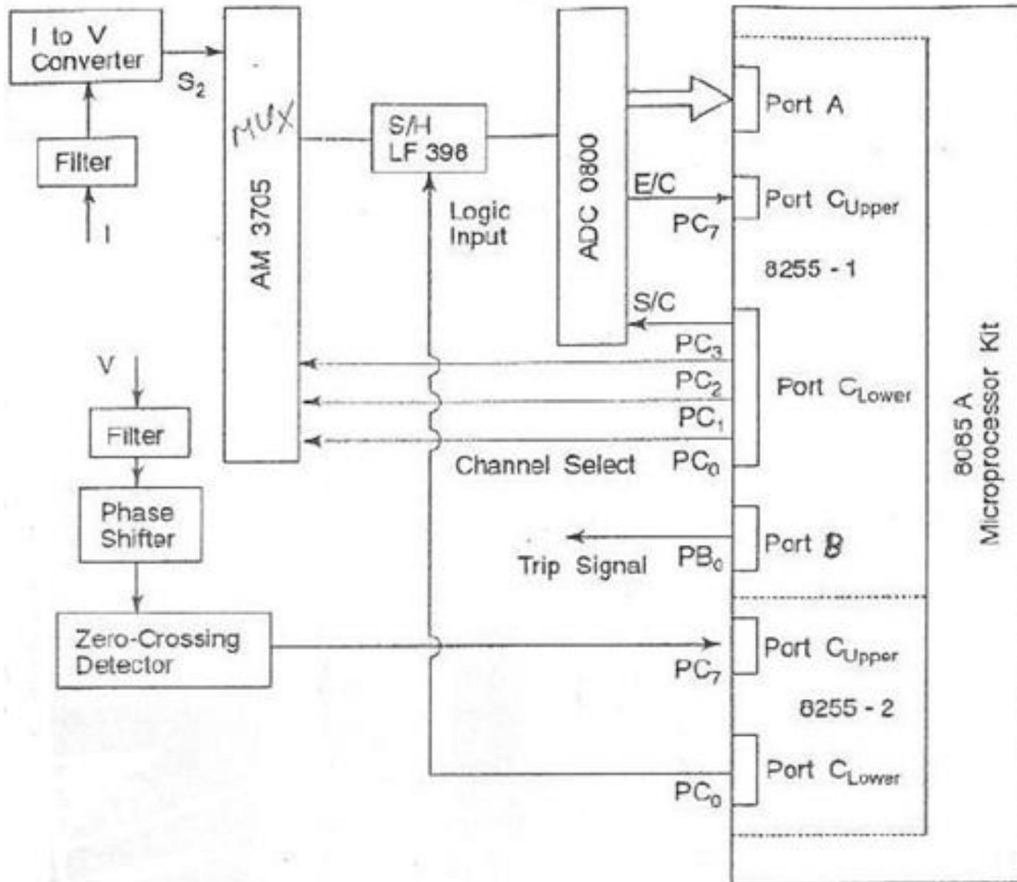
FIGURE 8.6 Block schematic diagram of interface for directional relay
