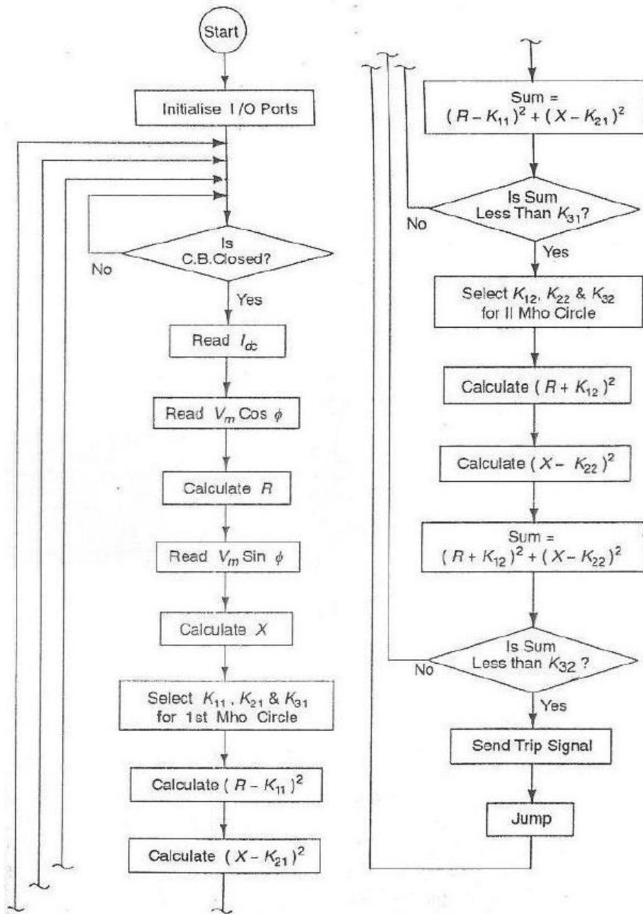
FIGURE 8.23 Program flowchart for restricted mho relay
