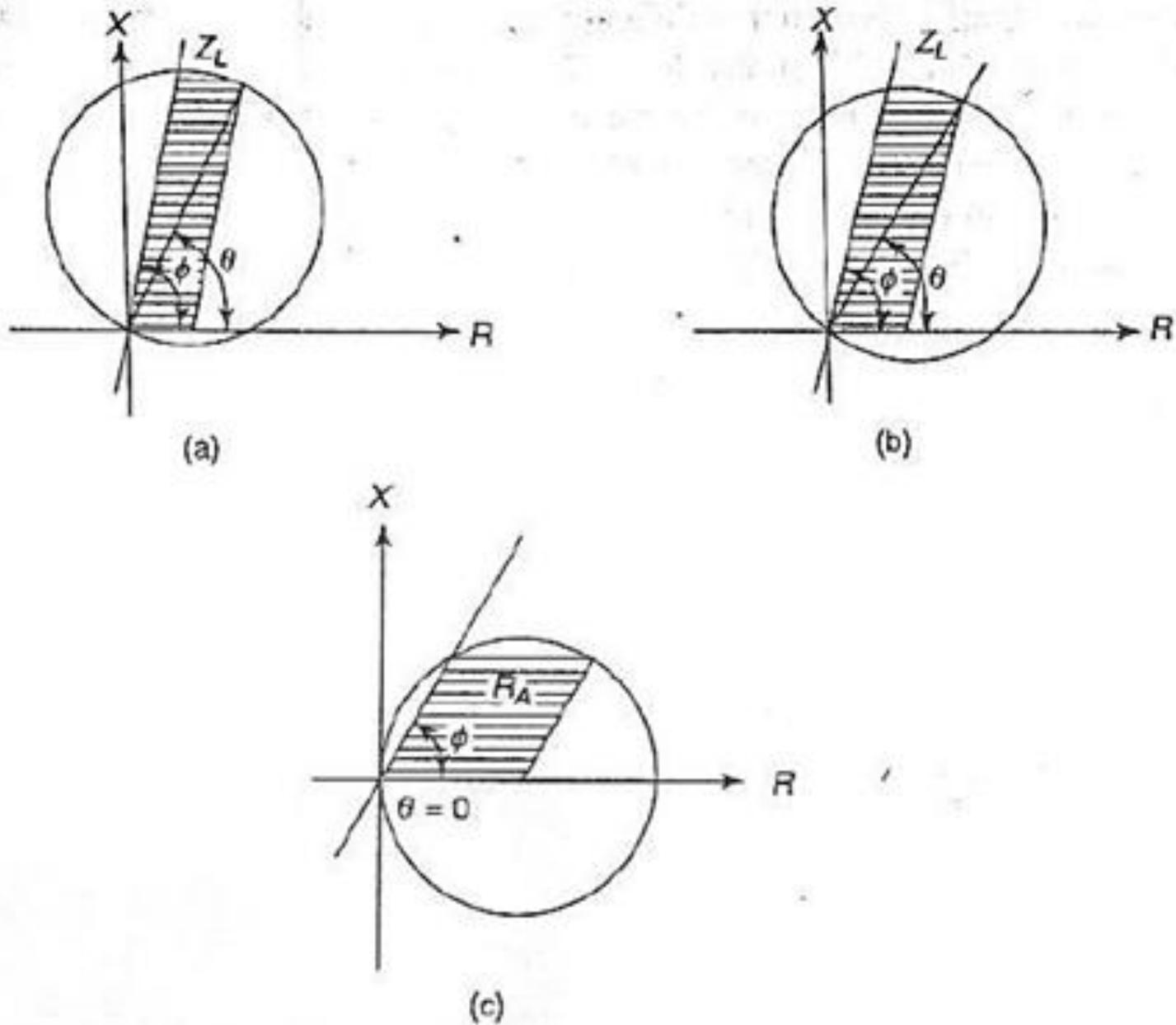
FIGURE 8.17 Mho relay's characteristics with different values of  $\theta$
