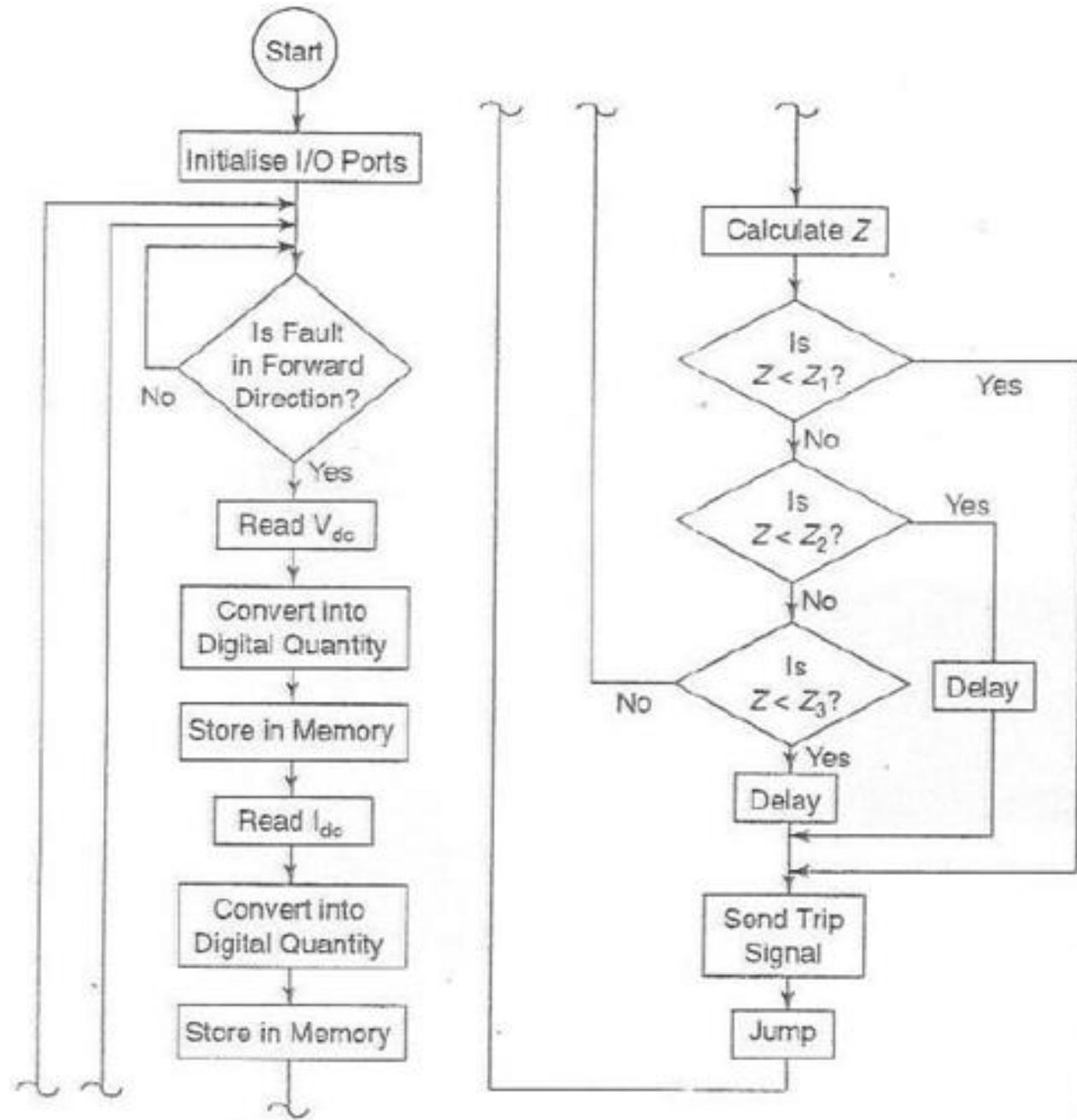
FIGURE 8.4 Program flowchart for impedance relay
