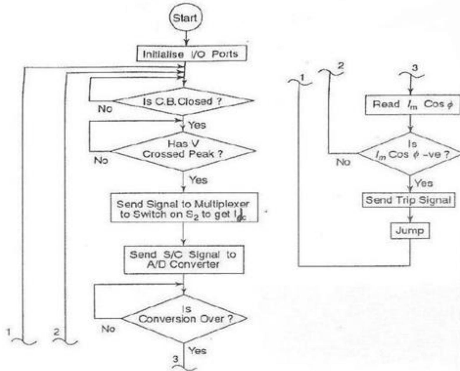
FIGURE 8.7 Program flowchart for reverse power relay
